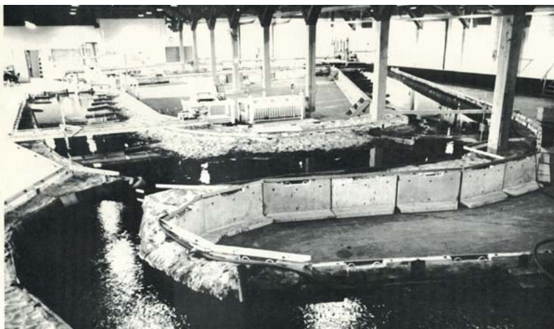
The Mead Hydraulic Lab at the ARDC was operated by the U.S. Army Corps of Engineers. The model was utilized to study the navigation channel at the junction of the Kansas and Missouri Rivers near Kansas City, Missouri. An interesting component of the project was that finely ground walnut shells were utilized to simulate Missouri River sand.
